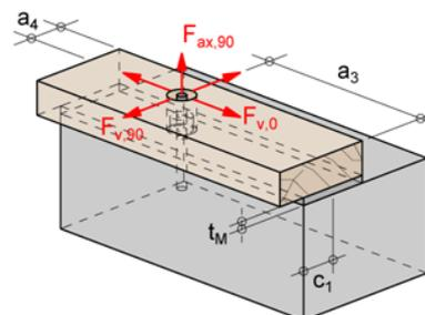
Fig. 3.1: Loading directions
