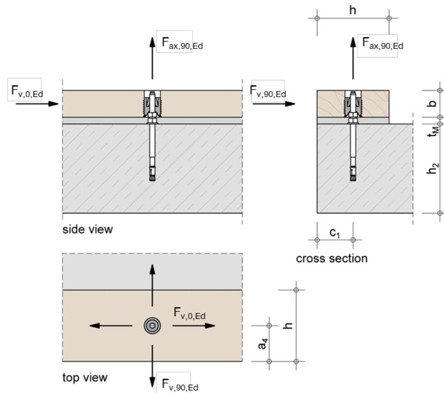
Fig. 6.1: Details of the connection
